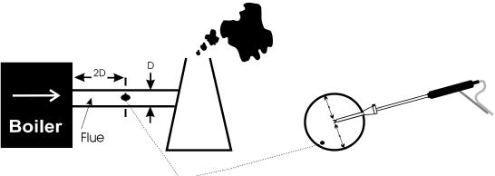
The probe depth stop cone provided with the instrument allows the probe to be used in holes whose diameters range from 8 mm to 21 mm ( $^{5}/_{16}$  to  $^{4}/_{5}$  inch).
