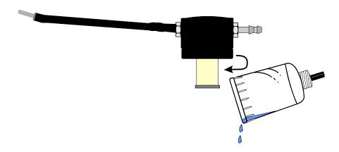
Carefully remove the end cap from the in-line housing. Dispose of the condensate in a suitable drain, care must be taken as it could be acidic. If condensate spills onto the skin or clothing, clean off immediately using fresh water, seek medical advice if problems occur.
