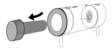
Remove the end cap from the filter housing. Carefully remove the paper filter element and dispose of it. Clean the inside of the filter housing with a suitable soft cloth. Insert a new filter element onto the spigot on the filter end cap and carefully insert it into the filter body.
